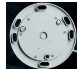
Installation The bottom plate of the SC 110 supports installation on structure using 3 or 4 x M12 on a 200 mm radius or 3 x M8 on a 150 mm radius.
