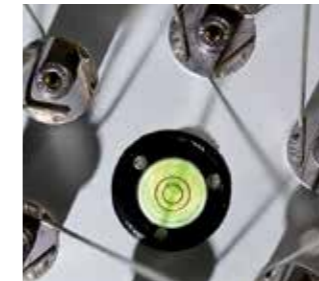
Level indicator The lantern can easily be levelled in field using the integrated bubble level indicator.
