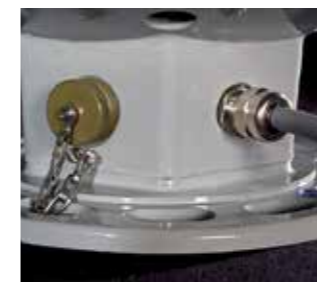
Additional cable entry Equipped as standard with two cable entries. If the second entry is needed e.g. for a solar module standard M20 cable gland can be fitted.
