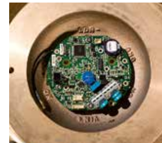
GPS GPS unit and antenna integrated in the lantern hat for wireless synchronization and for position monitoring. The integrated GPS antenna is moulded and survives ice pressure.
