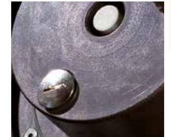
Additional cable entry Equipped as standard with two cable entries. If a second entry is needed, e.g. for a solar module, a standard M20 cable gland can be fitted.
