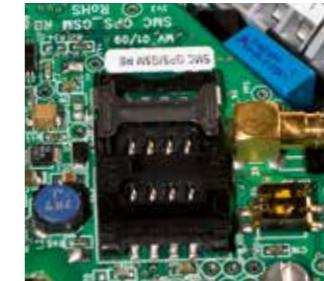
GSM GSM unit and antenna integrated in the lantern for remote monitoring and control. For more information please see the LightGuard Section.
