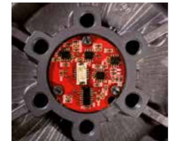
OFBS The Optical Feedback System (OFBS) enables built-in monitoring of LED degradation over time.
