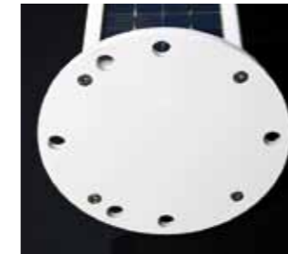
Installation The bottom plate of the M701-5 is machined powder-coated aluminium. It supports installation on structure using 3 x M12 bolts, 4 x M12 bolts, or 5 x M12 bolts on a 200 mm radius. Standard and security bolt kits are available.
