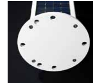
Installation The bottom plate of the M708 is machined powder-coated aluminium. It supports installation on structure using 3 x M12 bolts or 4 x M12 bolts on a 200 mm radius. Standard and security bolt kits are available.
